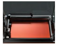
Preparation time is significantly reduced for all print projects by the fast-heating print bed. Capable of quickly reaching 100 °C for optimal print bed adhesion with a variety of high-quality materials. An inductive sensor enables semi-automatic print bed levelling to ensure optimal calibration and maximum control.
